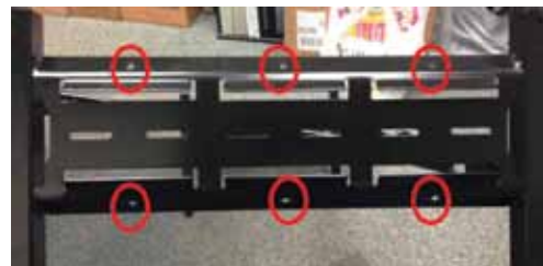
Cable tie holes to prevent pumps from falling off brackets
