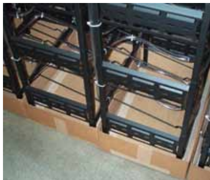
Racks are placed in corrugated top and bottom shells with bead board
